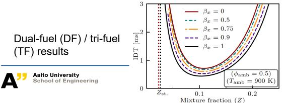
Therefore, adding H2 extends the operational window for methanol DF ignition
