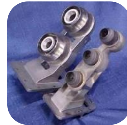
Premixed combustors Max \text{H}_2 ~10%
