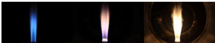
Images of flames from the high pressure combustion duct under different pressure ranges.
