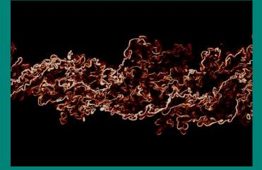
Scalar dissipation rate field in a turbulent mixing layer at high Reynolds number (A. Attili and F. Bisetti, Phys Fluids 24, 2012; Phys Rev E 88, 2013)
