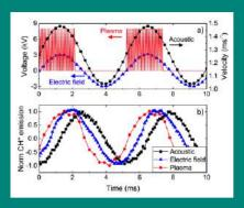
Forcing signals at 196 Hz and corresponding temporal evolution of normalized CH\* emission of M-flame.
