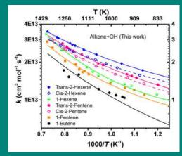
Rate coefficient of reaction of C4, C5 and C6 alkenes with OH radicals. Lines represent curve fits to data.
