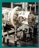
Shock tube used to measure reaction rates
