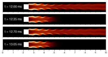
Temporal sequence of heat release rate isocontours for the syngas flames at U = 16.7 m/s, showing a periodic oscillation mode.
