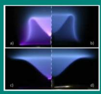
Methane-air M- and V-flames (b) & (d), forced by non-thermal plasma discharges (a) & (c)
