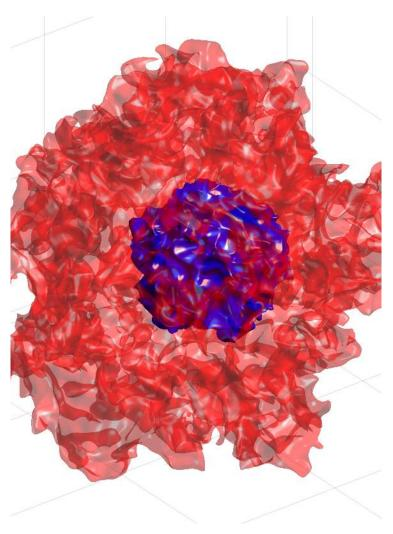
Visualization from a Direct Numerical Simulation of a spherical expanding turbulent methane flame at 4 atm (simulation performed by R. Buttay, S. Luca, A. Attili, F. Bisetti)
