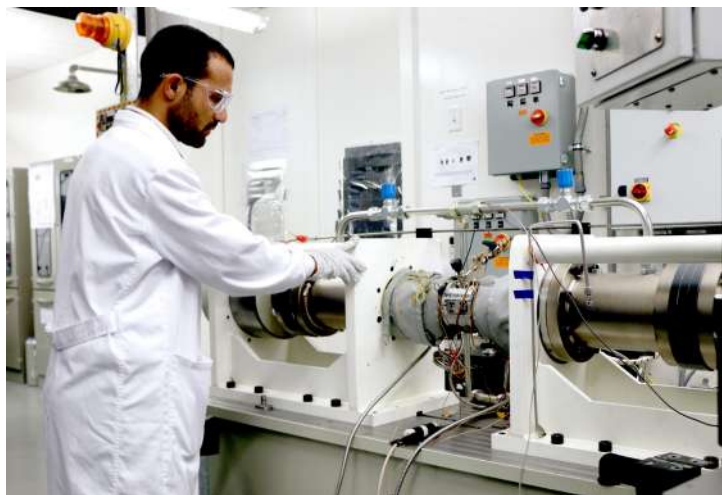
Figure 1: The Dual-ported Piston Rapid Compression Machine facility in the Chemical Kinetics and Laser Sensors Laboratory at KAUST
