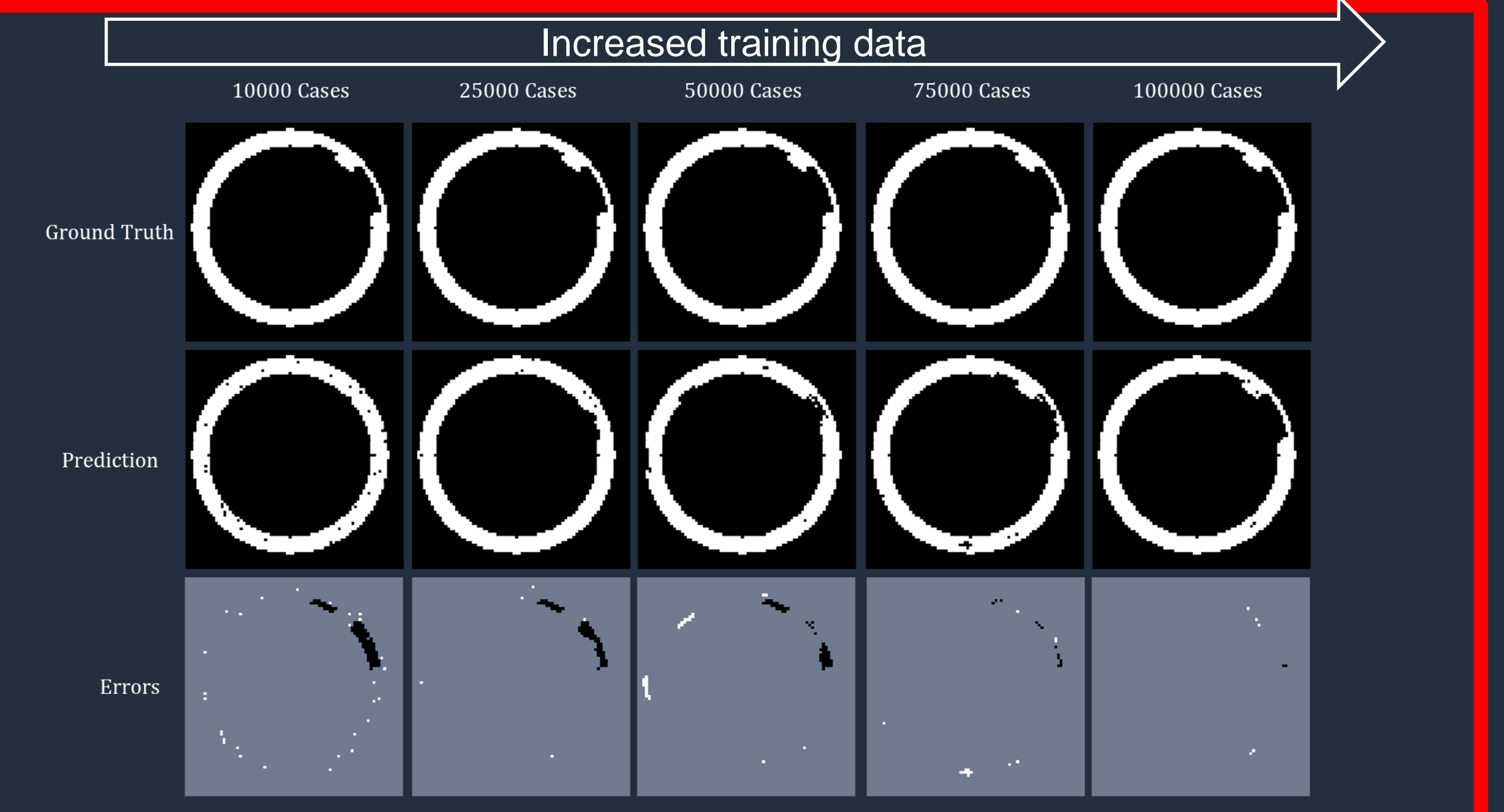
Cross-sectional inversion image of a pipe with the same defect, i.e. one record from the test dataset. Significant improvements in quality of prediction, middle column, in comparison to ground truth, top, as the amount of training data is increased, left to right. The difference errors plotted in the bottom panel
