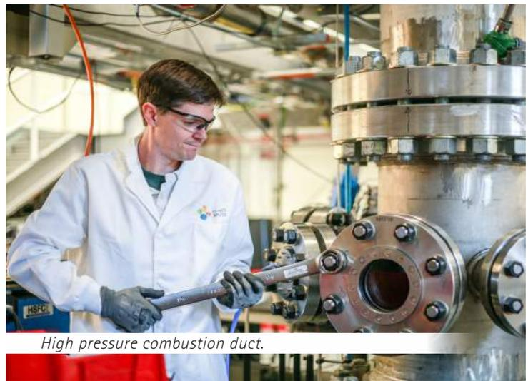
High pressure combustion duct.
