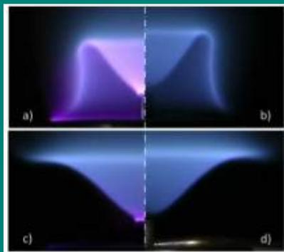
Methane-air M- and V-flames (b) & (d), forced by non-thermal plasma discharges (a) & (c)
