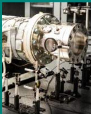
Shock tube used to measure reaction rates
