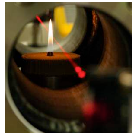
Laser Based Soot Measurement in a High Pressure Ethylene Coflow Diffusion Flame
